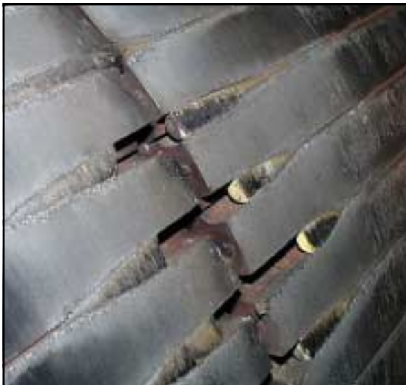
FIGURE 5: OPEN ROTOR BARS
