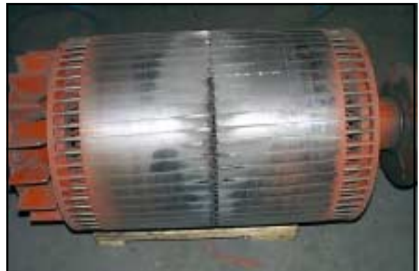
Fabricated copper alloy rotor with open bars that have worn through the tops of the slots.
