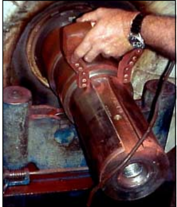
The same technique that can be used for ultrasonic testing of end rings is shown here being used on a shaft.
