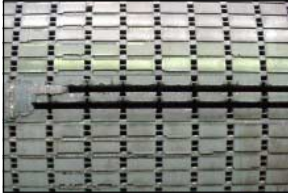
FIGURE 6: OPEN ROTOR BARS
