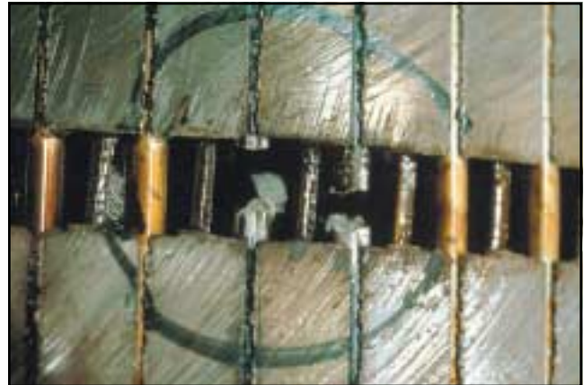
FIGURE 4: OPEN ROTOR BARS
