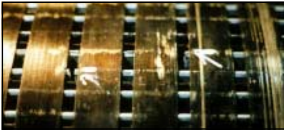
Open bars in a fabricated aluminum rotor.
